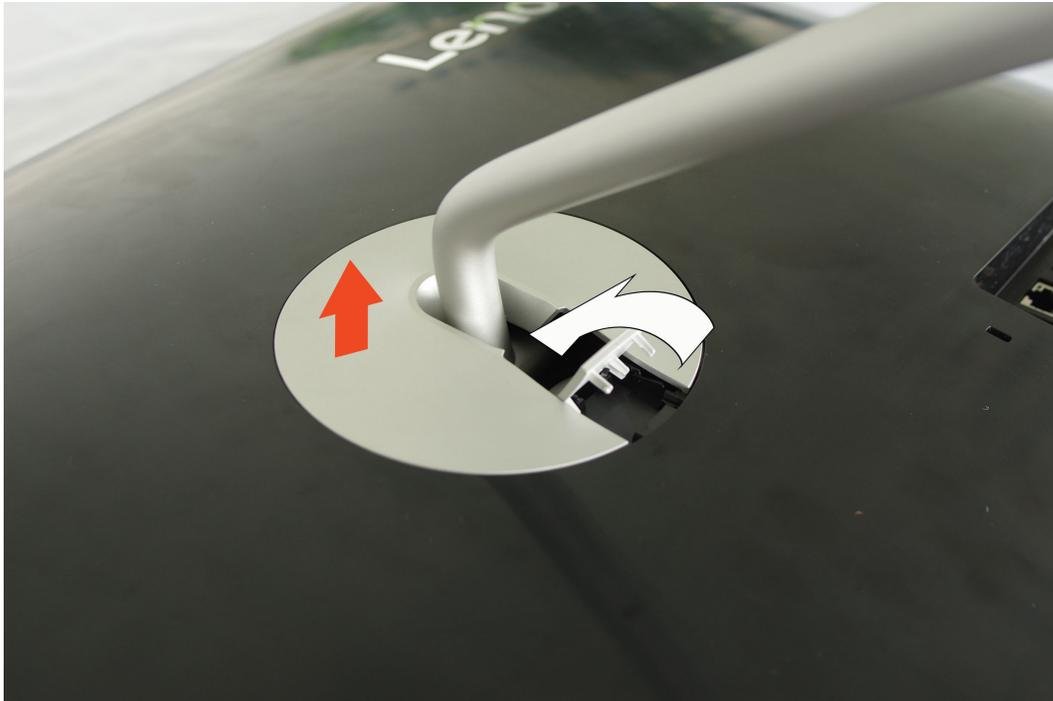
Step 6. Remove the screw cover rubber.
