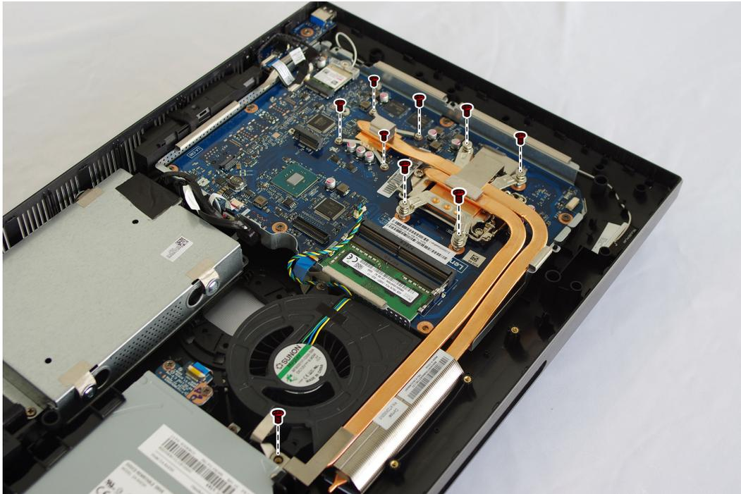
**Attention:** Place the heat-sink upside down on a flat surface to prevent thermal grease from contaminating other components.
