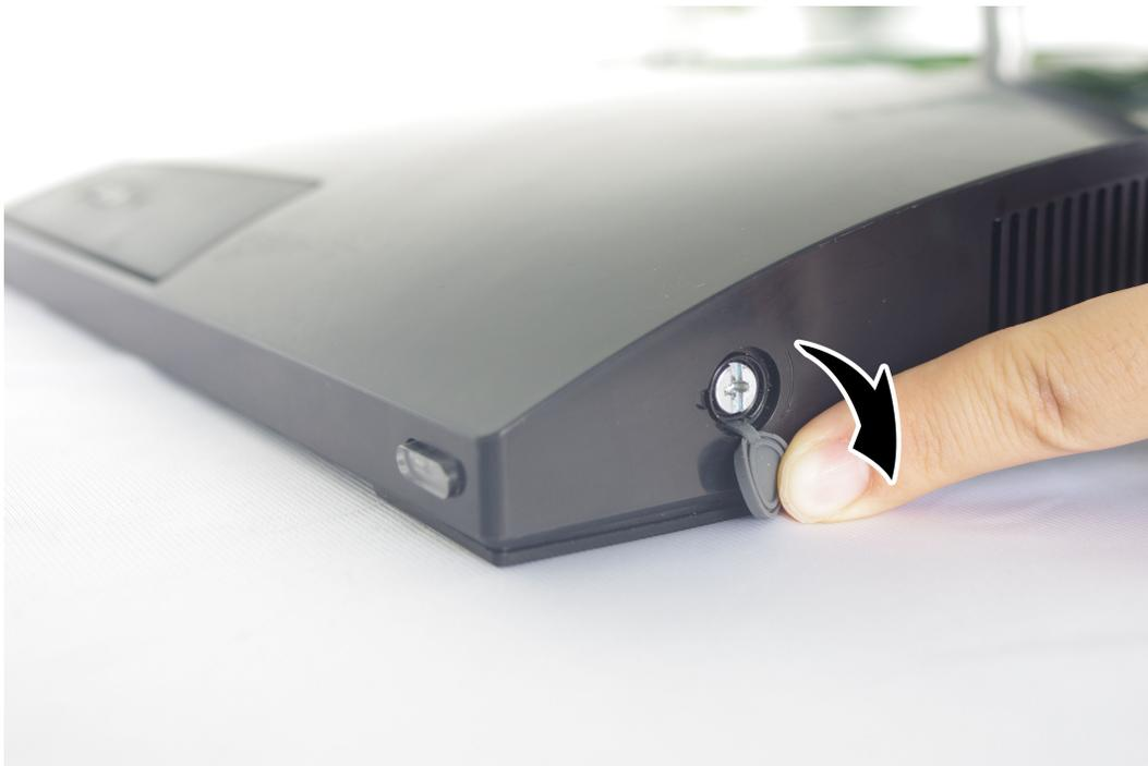
Step 7. Rotate the screwdriver 90 degrees to the right, and then lift up the rear cover from the left side bottom.
