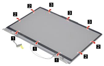
Figure 27. Remove the LCD bezel (on selected models)
