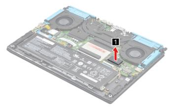
Figure 8. Remove the SSD thermal pad
