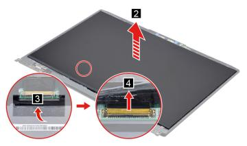
Figure 31. Disconnect the EDP cable and remove the LCD panel
