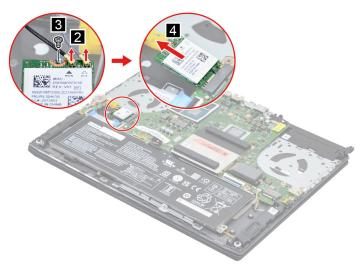
Figure 13. Remove the Wi-Fi card
