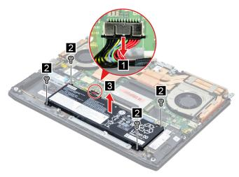
Figure 7. Remove the battery pack (on selected models)
