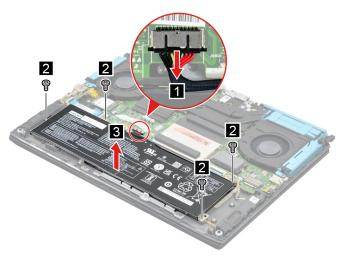
Figure 6. Remove the battery pack (on selected models)
