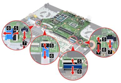
Figure 23. Disconnect cables connected to the system board
