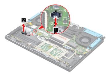
Figure 18. Remove the CMOS battery
