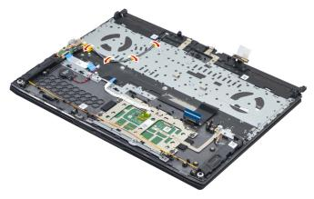
Figure 25. Release the antenna cable
