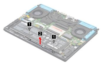
Figure 21. Remove the touchpad board bracket
