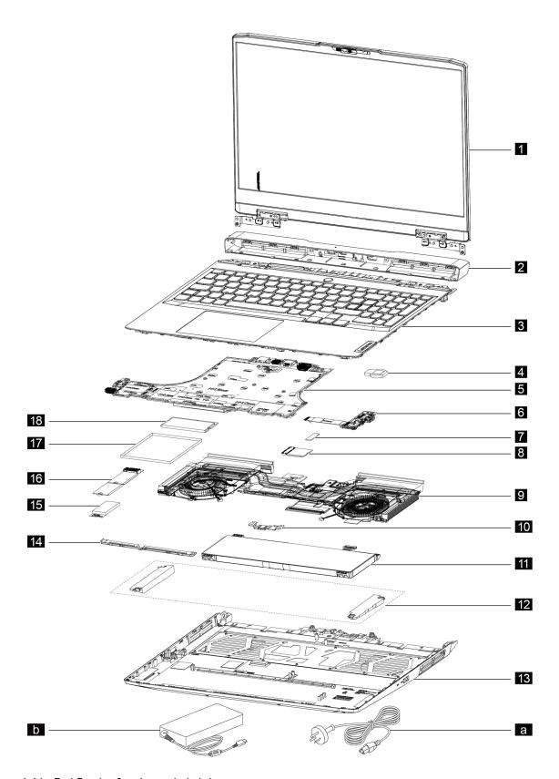
Figure 1. IdeaPad Gaming 3 series exploded view
