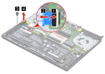
Figure 15. Remove the I/O board
