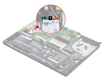
Figure 12. Remove the mylar
