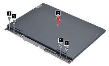
Figure 26. Lift the LCD module
