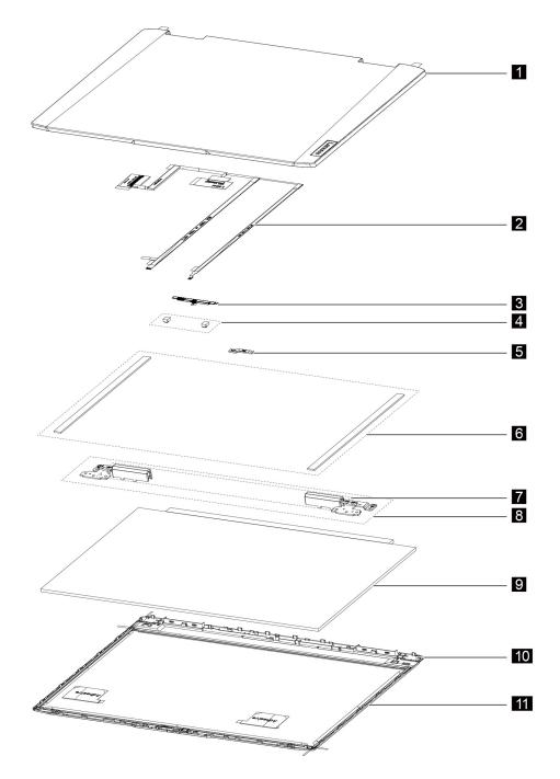
Figure 2. IdeaPad Gaming 3 series LCD module — exploded view
