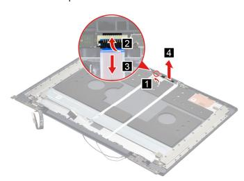
Figure 34. Remove the camera board
