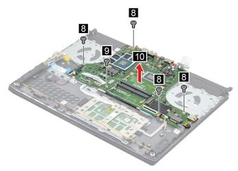
Figure 24. Remove the system board
