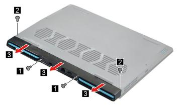
Figure 3. Remove four screws
