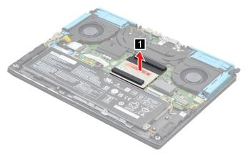
Figure 16. Remove the memory shielding
