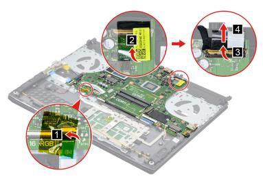
Figure 22. Disconnect the EDP cable connector
