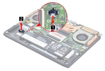
Figure 19. Remove the CMOS battery
