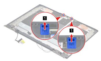
Figure 32. Remove the microphone rubbers
