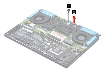
Figure 14. Remove the DC-in bracket
