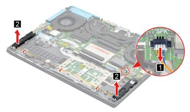
Figure 20. Remove the speakers
