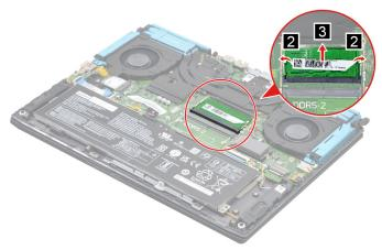
Figure 17. Open the buckles and then remove the memory
