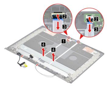
Figure 35. Remove the EDP cable
