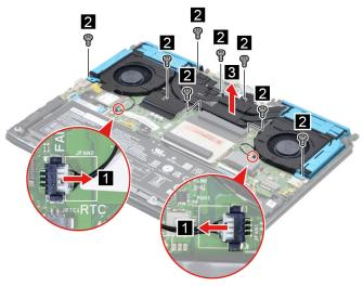
Figure 11. Remove the thermal module
